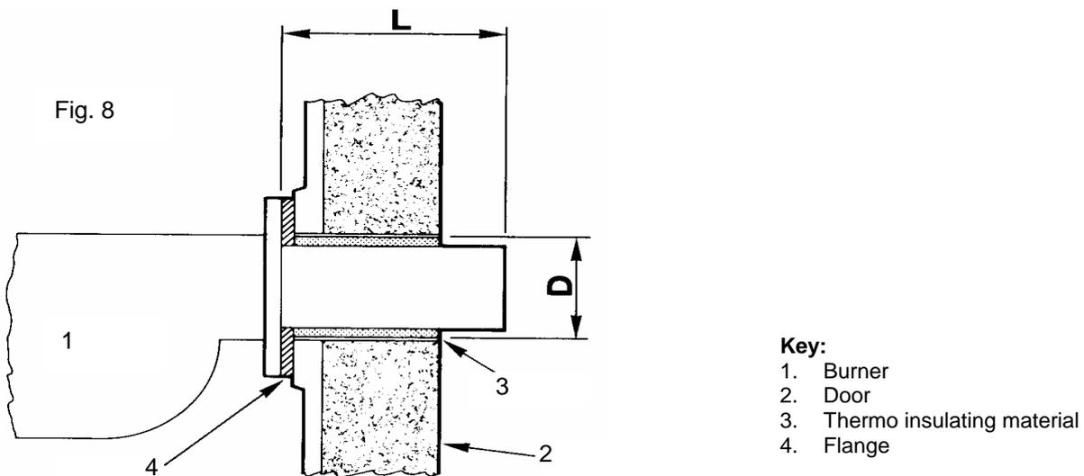
Verify that the spaces between the burner sleeve and the boiler door are suitable filled with flame-resistant ceramic insulation (Fig. 8).
